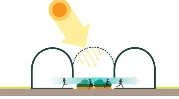
ABOVE A net roof creates a shaded outdoor room at the centre of the school. This allows for exterior play and farming activities, as well as free movement between the two large interior spaces on either side.
