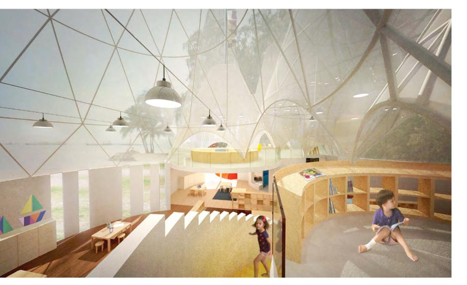
LEFT A Teflon-coated fabric enclosure allows filtered natural light to partially illuminate the learning spaces.
